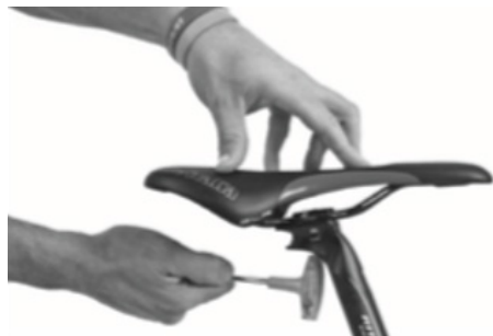
Loosen both screws with about two or three turns.
