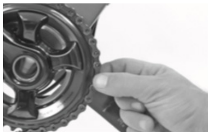
Check of the chain conditions.
