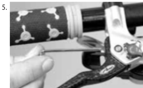
Setting of distance between brake lever and handlebar.
